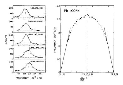
Fig. 16: Kohn Effect in dispersion curves of Pb [53]. (a) A series of closely-spaced phonons show anomalous variation (b) in the corresponding dispersion relation v(q), in this case at a calliper dimension of the Fermi surface in the  $[\zeta,\zeta,\zeta]$  direction.
