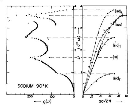
Fig. 17. The frequency distribution g(v) for Na at 90 K [55], calculated from a force constant model fitting the dispersion curves v(q) also shown [54]. The relation between the frequencies at symmetry points and the Van Hove [14] singularities in g(v) are exhibited.
