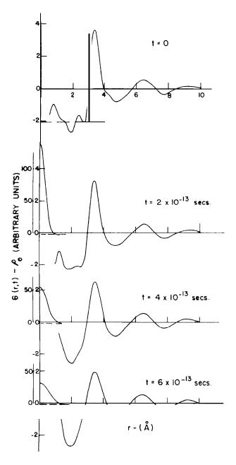
Fig. 8: Van Hove transformations of the data of Fig. 8 [34]. The distribution for time t=0 is essentially the familiar pair distribution of X-Ray scattering experiments. The peak ( $\delta$ -function) at the origin gradually diffuses outwards with elapsed time t as do the first and subsequent neighbour peaks in a sort of moving picture of what goes on in the liquid.
