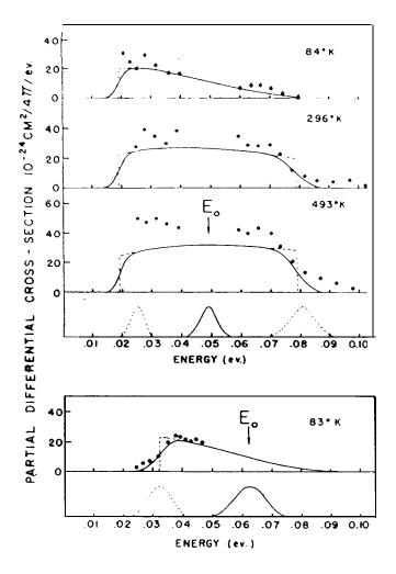
Fig. 4b: The transformed energy distributions (points) of the inelastic component in vanadium (Fig. 4). The curves are calculated (one-phonon) cross-sections for a Debye frequency distribution for the lattice vibrations. The elastic component provides a measure of the resolution function at the incident energy.
