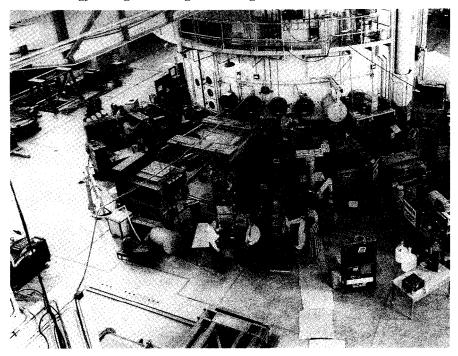
Fig. I: The main floor of the NRX Reactor at the Chalk River Laboratory about 1950. The powder diffractometer constructed by Donald Hurst and associates is visible near the centre of the photograph. Most of the other equipment is concerned with nuclear physics or with the physics of the neutron itself. For reasons of space, each apparatus is located at the end of a long tube. (AECI. photo)
