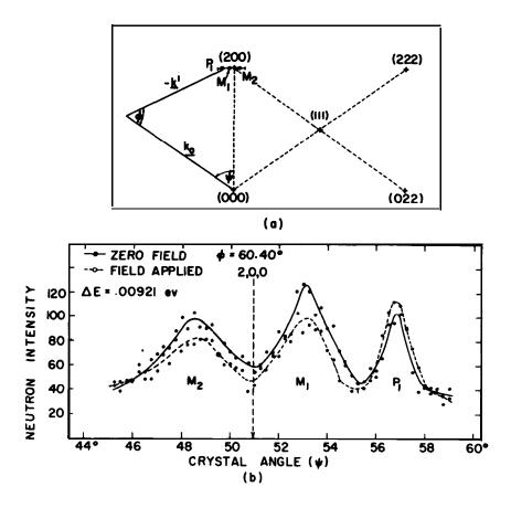
Fig. 12: Momentum diagram (a) and neutron groups (b) for a crystal of (F.C.C.) Co (8% Fe). The magnetic signatures on the intensities indicate that M, and M, are groups for spin wave quanta (magnons) and that P, is a phonon group [41].
