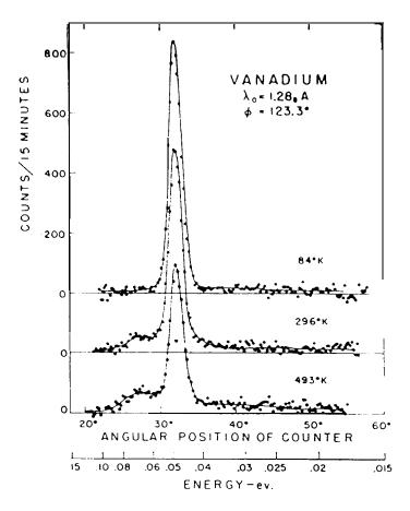
Fig. 4a: Measured energy distributions of neutrons scattered by vanadium as functions of the angular settings of the analyzing spectrometer, for three temperatures, with backgrounds substracted and intensities normalized [27]. The intensity of the elastic peak decreases with temperature in about the manner expected from Debye-Waller theory. The inelastic component is affected by the extreme dispersion of neutron spectrometers and requires transformation to a true energy distribution.
