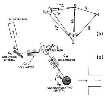
Fig. 10: Schematic drawing of a triple-axis spectrometer together with the momentum space diagram in the same co-ordinate system. The dashed lines indicate a second point on a "Constant Q" curve at fixed incoming energy [43]. The massive shielding required, particularly around the monochromator, is not shown.
