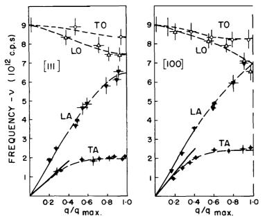
Fig 13: Dispersion curves for germanium at room temperature, showing optical and acoustic branches in two symmetry directions [45].
