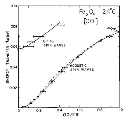
Fig 11: Dispersion curves for spin waves in a magnetite (Fe,O,) crystal [40], showing the expected initial quadratic behaviour and the initial part of an optical mode.
