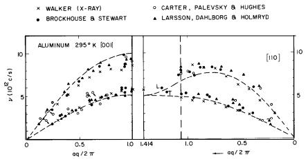
Fig. 6: Dispersion curves for aluminium at room temperature, for two symmetry directions in the crystal (collected results [28 – 30]. The neutron measurements from three laboratories are consistent with each other within the errors and are almost so with those inferred [18] from intensities of scattered X-Rays. Nevertheless the discrepancies would be very important in attempts to extract inter-atomic forces from the data
