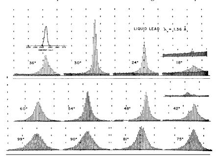
Fig. 7: Histogram, [43] of energy-analyzed distributions of neutrons scattered by liquid lead at a series of scattering angles [34]. The scattering angles are roughly related to the momentum transfer Q the abscissa angles to the energy transfer. Appropriate measured backgrounds are also given. The resolution function measured with a vanadium scatterer is shown at the upper left.
