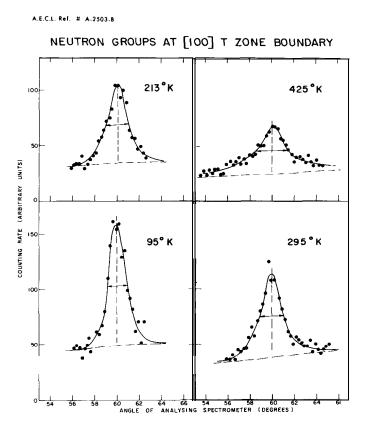
Fig. 15: Neutron groups for a symmetry phonon in a crystal of Pb at four temperatures showing line-widths increasing with temperature [60]. This receives a natural interpretation as a reduction with temperature of the lifetime and coherence length of the phonon involved, because of interaction with other phonons.
