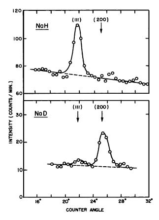
Fig. 5: Patterns for NaH an NaD Showing that Hydrogen Contributes Normally to the Pattern.
