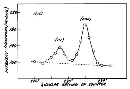
Fig. 4: Portion of the First Powder Difraction of NaCl taken at the Clinton Pile. I
