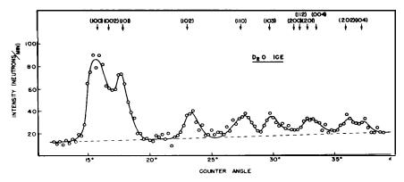
Fig. 6: Pattern Taken for a Sample of Powdered D<sub>2</sub>O Ice.
