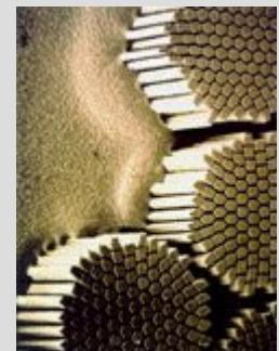
CERN, LHC Machine Outreach: Super conducting cable,
