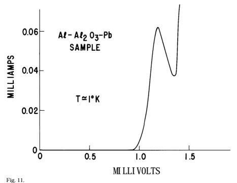
A negative resistance characteristic obtained experimentally in tunneling between two different superconductors.
