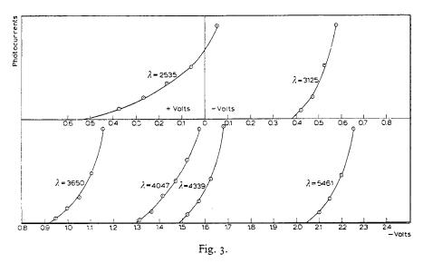
narrow limits of experimental error, of the Einstein equation, and the first direct photoelectric determination of Planck's h. The accuracy obtained was about 0.5% which was much the best available at the time. Figs. 3 and 4, which represent the most accurate work done on an individual metal (so-dium), will illustrate the entire lack of ambiguity of the result.
