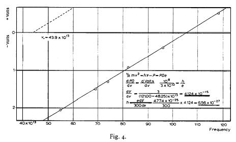
D. L. Webster<sup>9</sup> then proved that the characteristic X-ray frequencies of atoms begin to be excited at just the potential at which the energy of the stream of electrons which is bombarding the atoms has reached the value given by  $hv = \frac{1}{2}mv^2$  in which *v* is now the frequency of an absorption edge.
