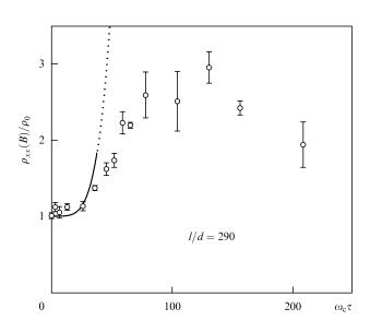
**Figure 4.** Magnetoresistivity in a random potential from computer simulations in comparison with Eqn (11).
