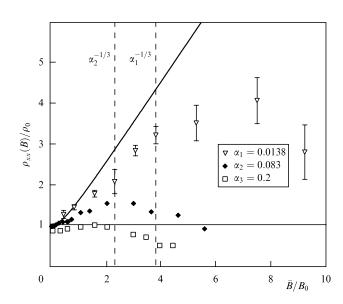
**Figure 3.** Magnetoresistivity (normalized by the Drude value) in a random magnetic field from numerical simulations for three different strengths of disorder; the full line corresponds to Eqn (10). Parameter  $\alpha = (d/2t)^{1/2}$ .
